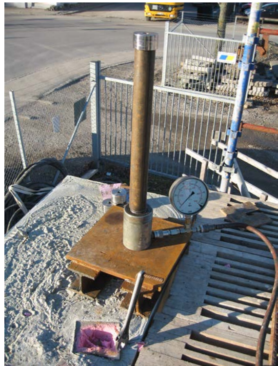
Figure A.5: Diaphragm wall after casting and excavation (top), drilling of concrete cores in a diaphragm wall panel (left), experimental assembly for pull-out test on the reference panel (right)
