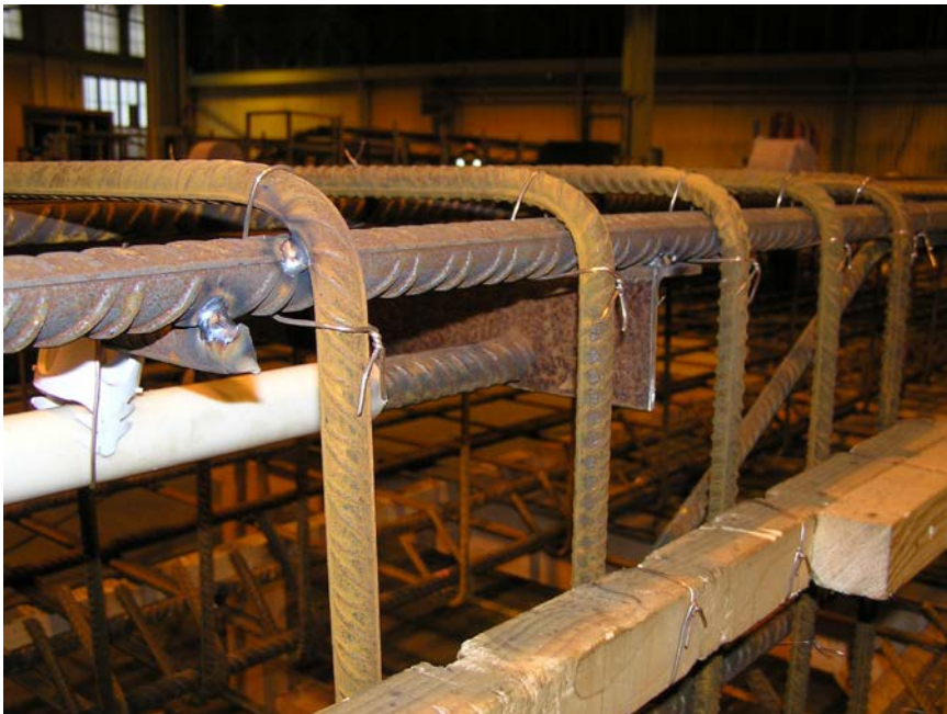
Figure A.2: Part of the bar to be embedded in the concrete for pull-out test
