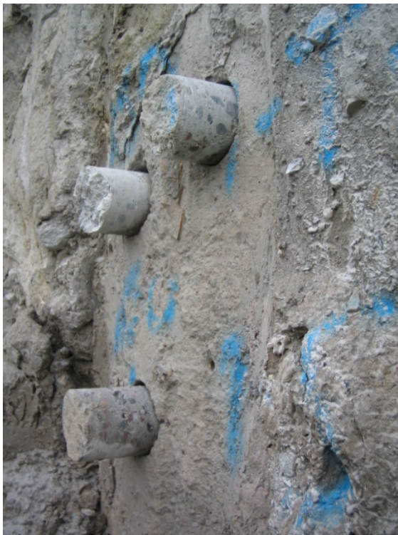
Figure A.5: Diaphragm wall after casting and excavation (top), drilling of concrete cores in a diaphragm wall panel (left), experimental assembly for pull-out test on the reference panel (right)
